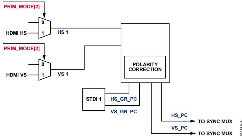
Figure 40. External/HDMI Syncs Routing to CP Section
