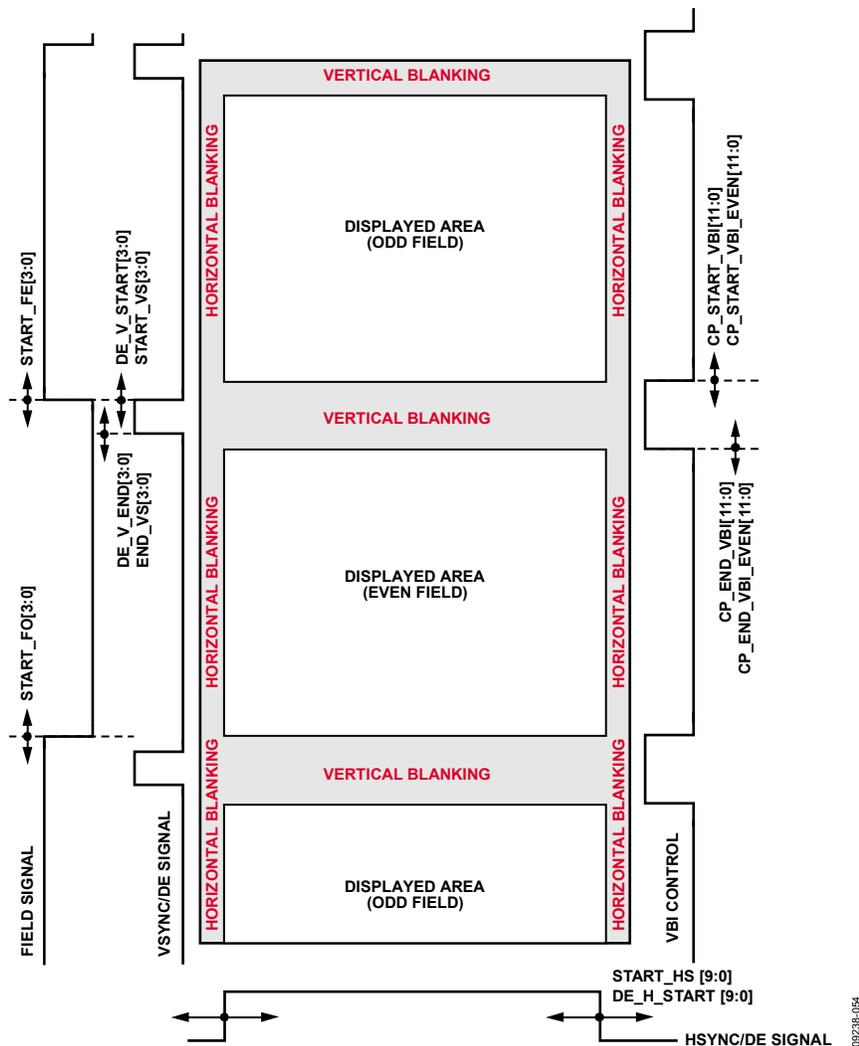
Figure 48. Synchronization Repositioning and Displayed Area
