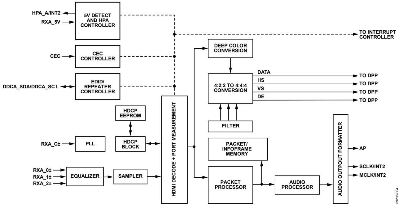
Figure 3. Functional Block Diagram of HDMI Core
