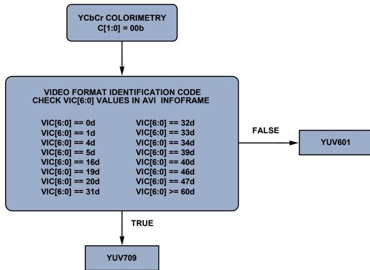
Figure 31. HDMI Auto CSC Flowchart (Case YCbCr-2)
