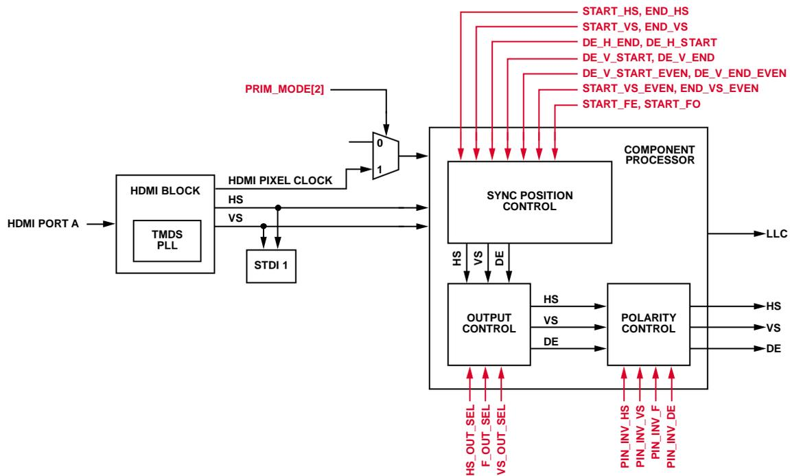
Figure 47. **ADV7611** Simplified Synchronization Signal Processing Flow Diagram
