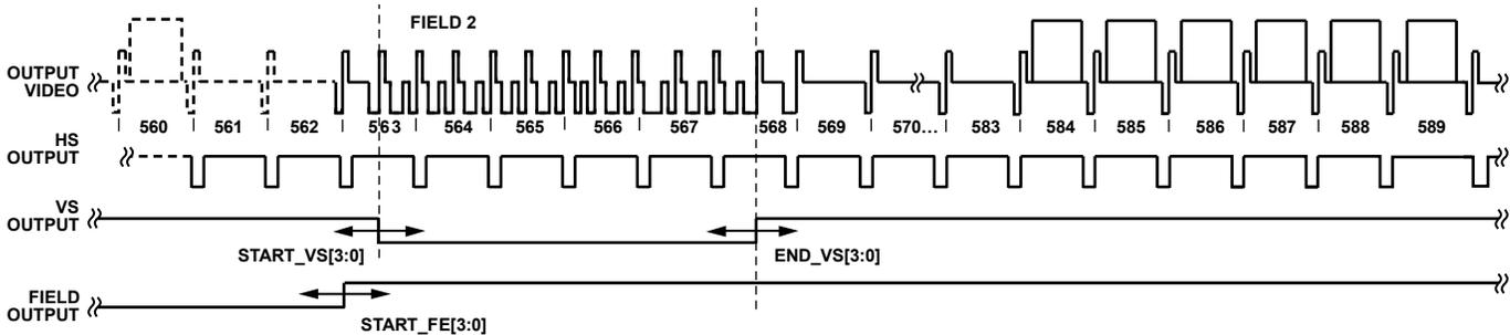
Figure 56. 1080p VS Timing
