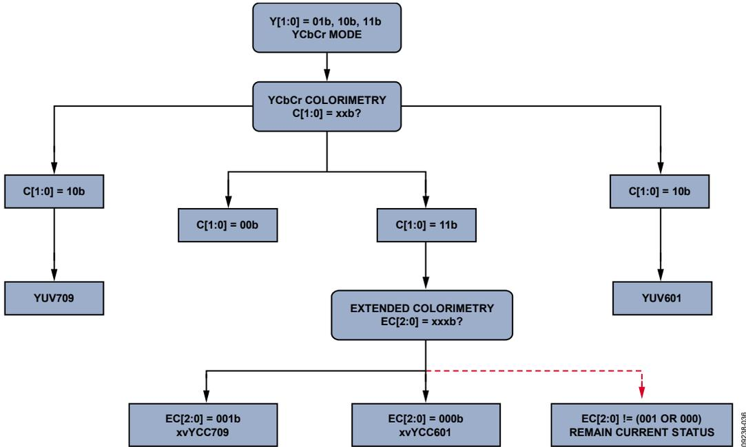
Figure 30. HDMI Auto CSC Flowchart (Case YCbCr-1)
