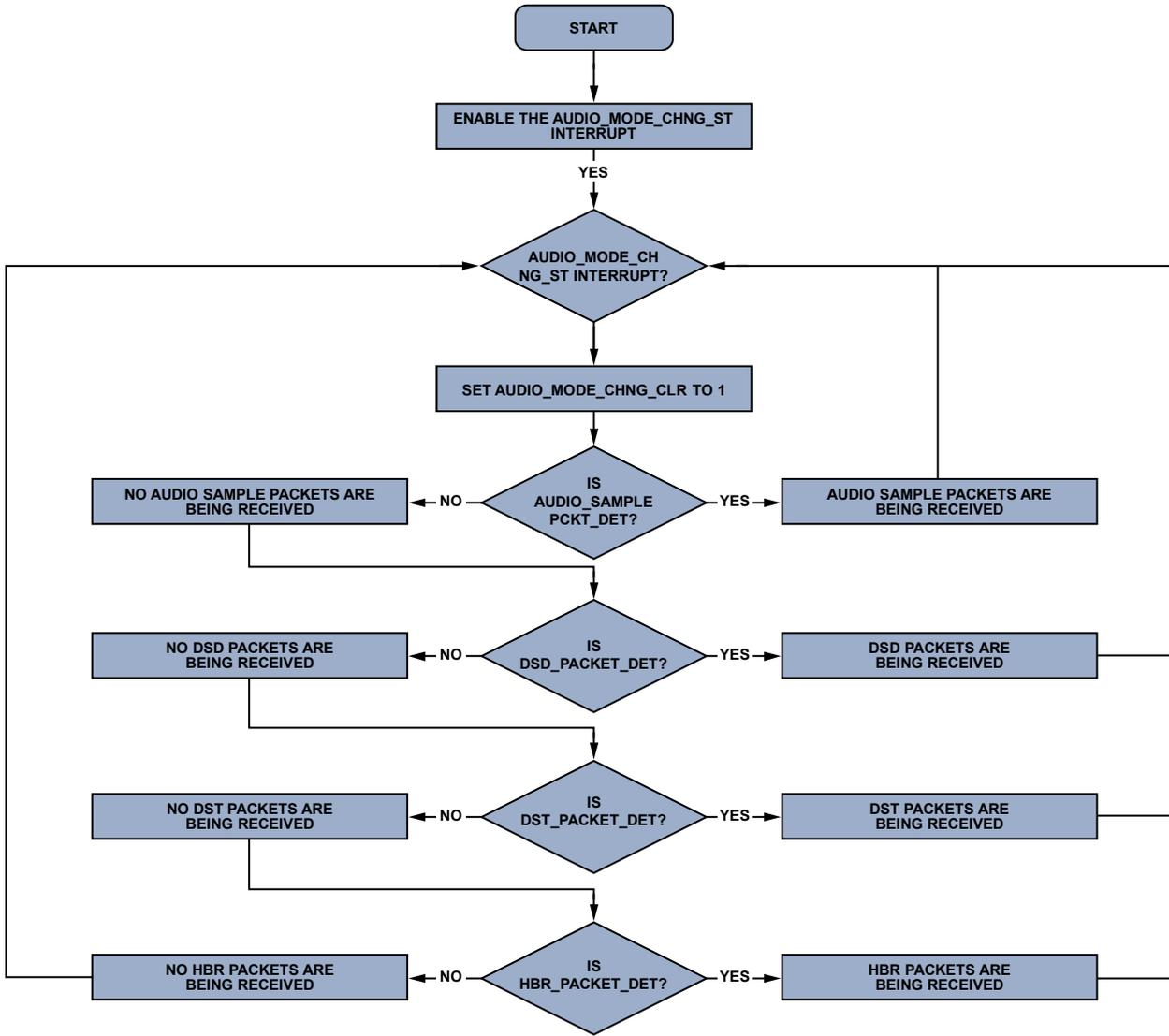
Figure 14. Monitoring Audio Packet Type Processed by ADV7611
