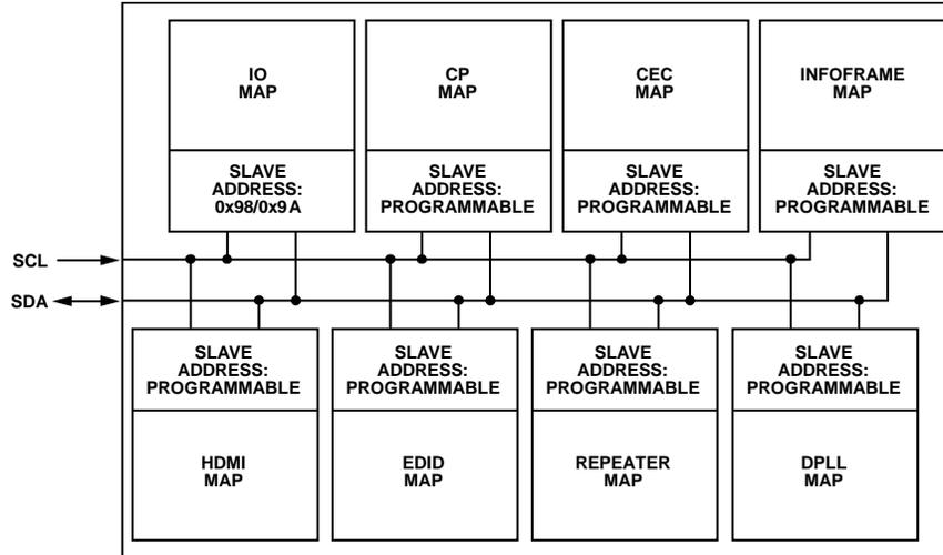
Figure 65. ADV7611 Register Map Access through Main I<sup>2</sup>C Port
