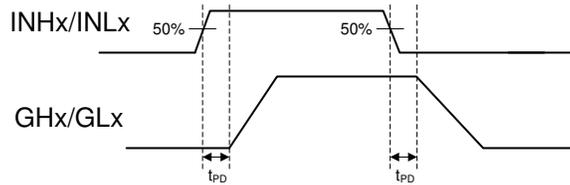
Figure 7-1. Propagation Delay (t<sub>PD</sub>)
