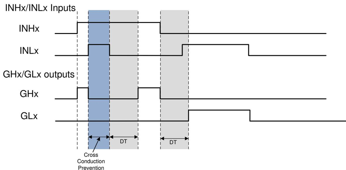
**Figure 8-3. Cross Conduction Prevention and Deadtime Insertion**
