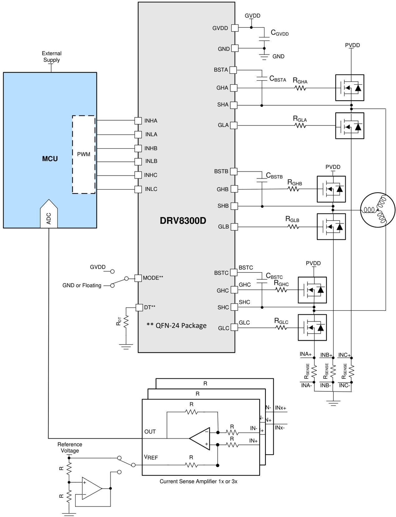
**Figure 9-1. Application Schematic**
