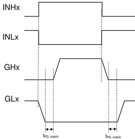
Figure 7-2. Propagation Delay Match (t<sub>PD\_match</sub>)
